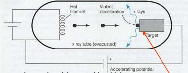
X-rays can be produced by smashing highspeed electrons into a metal target. When they hit, these decelerating charge produce much radiation, called...
