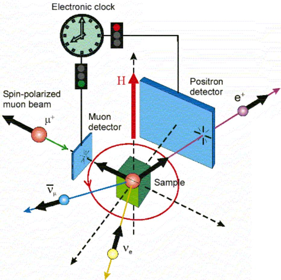
Field applied  $\perp$  to initial spin polarization
