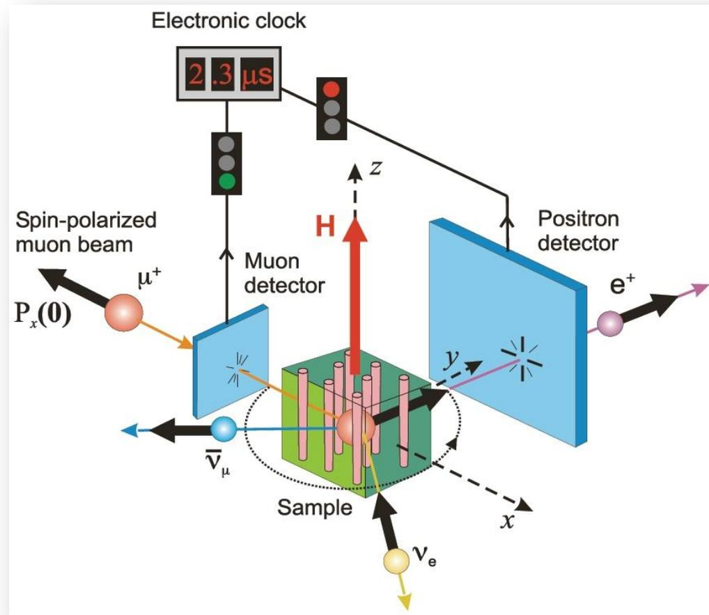
Field applied  $\perp$  to initial spin polarization
