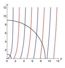
$$\begin{array}{ll} \eta = \rho \tan \rho & \text{even eigenfunctions} \\ \eta = -\rho \cot \rho & \text{odd eigenfunctions} \\ \rho^2 + \eta^2 = \frac{m V_0 L^2}{2 \hbar^2} & \text{constraint} \end{array}$$
