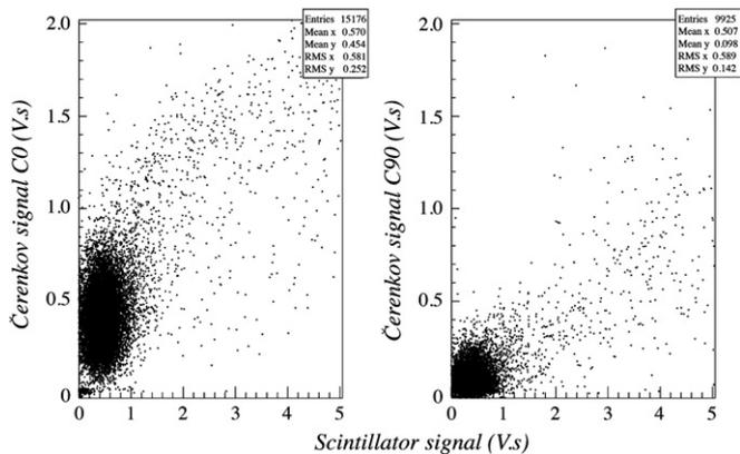
**Fig. 12.** Scatter plots relating the signals observed at the two ends of the crystal for 180 GeV  $\pi^+$  pions crossing the crystal at  $\theta = 30^\circ$ . Results are given for measurements in which the transmission axis of the polarization filter was oriented in the horizontal plane (a) and in the vertical plane (b).
