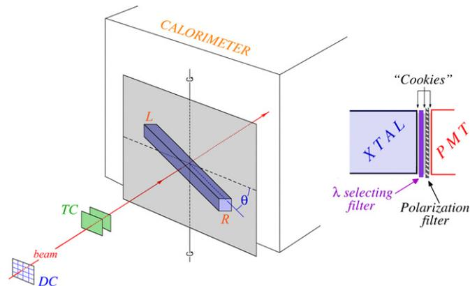
**Fig. 1.** Experimental setup in which the beam tests of the crystals were performed. The angle  $\theta$  is negative when the crystal is oriented as drawn here. Also shown is the coupling between the crystal and the readout element (PMT). These drawings are schematic and *not* to scale.
