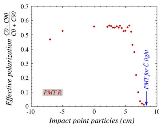
Fig. 7. The effective polarization of the Cherenkov light produced by 180 GeV  $\pi^+$  beam particles traversing the BSO crystal at  $\theta = 30^\circ$ . See text for details.
