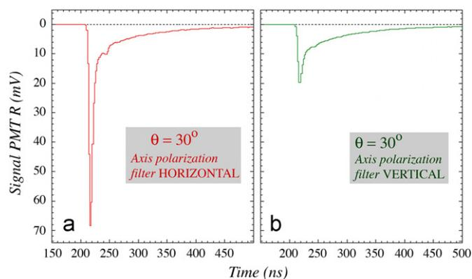
Fig. 5. Average time structure of the signals generated by 180 GeV  $\pi^+$  traversing a BSO crystal in its center at  $\theta = 30^\circ$  and passing through a U330 optical transmission filter, followed by a polarization filter. The transmission axis of the latter filter is either oriented horizontally (a) or vertically (b). The zero of the time scale is given by the start of the time base of the oscilloscope.
