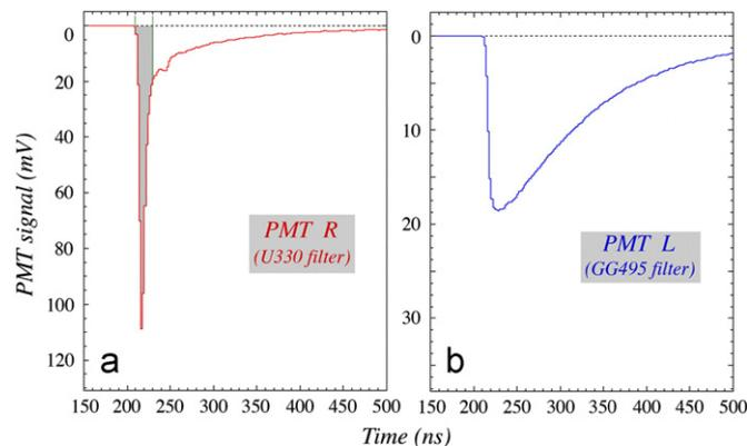
**Fig. 3.** Time structure of the signals generated by 180 GeV  $\pi^+$  traversing a BSO crystal in its center at  $\theta = 30^\circ$  and passing through a U330 optical transmission filter (a), or a GG495 yellow filter (b). The time scale describes the time passed since the start of the time base of the oscilloscope. The reflection observed in the signals from PMT R is caused by impedance mismatching.
