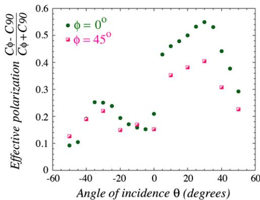
**Fig. 10.** The effective polarization of the Cherenkov light produced by 180 GeV  $\pi^+$  beam particles traversing the BSO crystal, as a function of the angle of incidence  $\theta$ , in the center of the crystal. Results are given for a rotation of the transmission axis of the polarization filter by  $90^\circ$  with respect to the vertical plane (maximum polarization) and for a rotation by  $45^\circ$ . See text for details.
