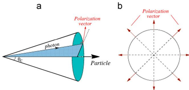
**Fig. 2.** Polarization of Cherenkov light emitted when a charged particle traverses a medium with refractive index  $n$  at a speed in excess of  $c/n$ . The light is emitted in a cone with angle  $\theta_c = \arccos[(\beta n)^{-1}]$  (a) and is polarized with the polarization vector oriented perpendicular to this cone (b).
