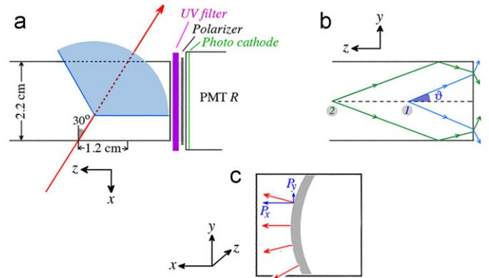
**Fig. 4.** Emission of Cherenkov light by particles traversing the BSO crystal at  $\theta = 30^\circ$ . Shown are a top view (a), a side view along the direction of the incident beam particles (b) and a view from the end face from which the Cherenkov photons exit the crystal (c). The Cherenkov cone is indicated by the shaded area in (a), and the polarization vectors of the detected Cherenkov photons by the arrows in (c). See text for further details.
