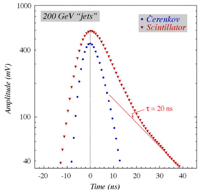
Fig. 5. The average time structure of the Cherenkov and scintillation signals recorded for 200 GeV “jets” in the fiber calorimeter.
