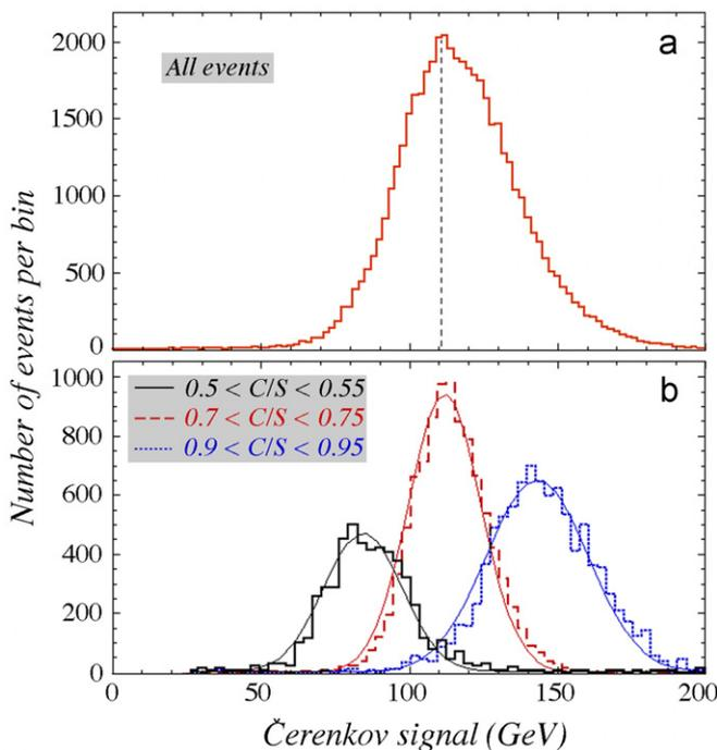
Fig. 4. The Cherenkov signal distribution for 200 GeV “jet” events detected in the BGO + fiber calorimeter system (a) together with the distributions for subsets of events selected on the basis of the ratio of the total Cherenkov and scintillation signals in this detector combination (b).
