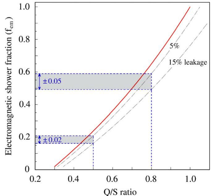
**Fig. 2.** The relationship between the  $Q/S$  signal ratio and the em shower fraction,  $f_{em}$  (Eq. (3)). Also shown is how a shower leakage of  $10 \pm 5\%$  translates into an uncertainty in the em shower fraction.
