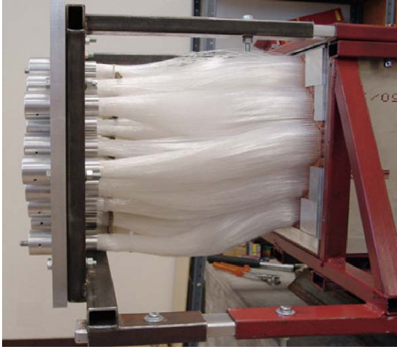
Fig. 3. Fiber bunches exiting from the rear face of the DREAM calorimeter. Each bunch was tightly squeezed by means of a thin metal collar with adjustable radius. In the following, we refer to these squeezed fiber bunches as “ferrules”.
