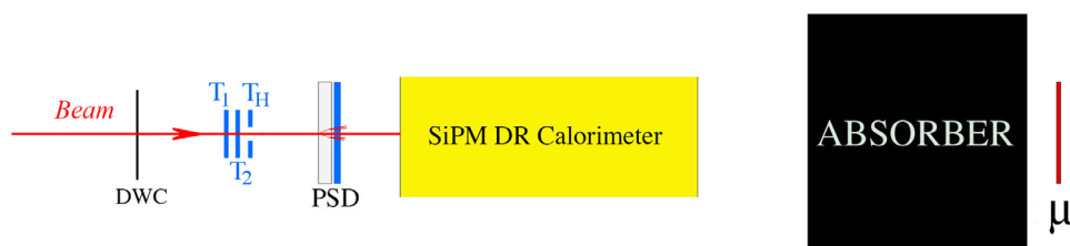
Fig. 6. Schematic layout of the experimental setup (not to size). Shown are the delay wire chamber (DWC), the trigger counters (TC), the preshower detector (PSD) and the muon counter ( \mu ).
