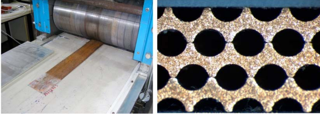
Figure 26: The machine with which the 1 mm thick copper foils are being rolled into the desired shape, and the result of this process.
