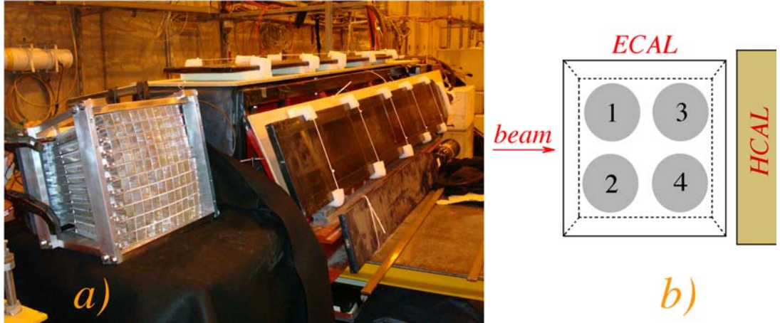
Figure 15: The calorimeter during installation in the H4 test beam, which runs from the bottom left corner to the top right corner in this picture. The 100-crystal BGO matrix is located upstream of the fiber calorimeter, and is read out by 4 PMTs on the left (small end face) side. Some of the leakage counters are visible as well (a). The location and numbering of the PMTs reading out the BGO crystal matrix (b) [17].
