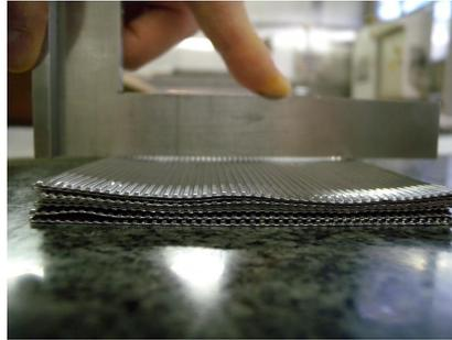
Figure 64: The "S" shape of the lead plates, caused by the non-uniformity of their thickness.
