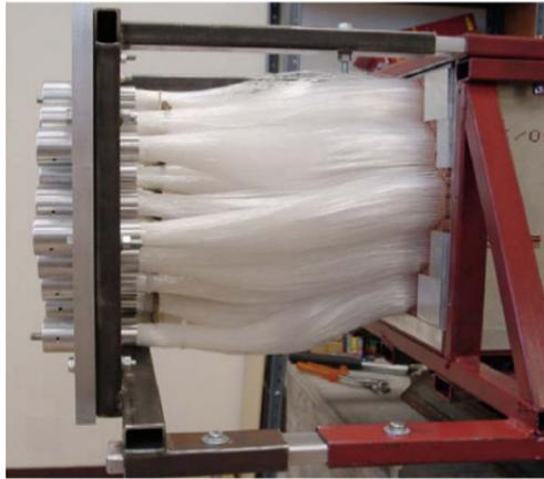
**Figure 34:** Fiber bunches exiting from the rear face of the DREAM calorimeter. Each bunch was tightly squeezed by means of a thin metal collar with adjustable radius. [13]
