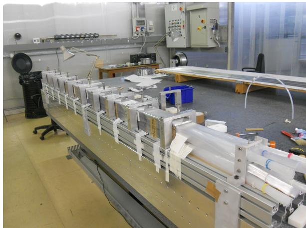
**Figure 62:** A picture of the module fixed and pressed by clamps for the night.
