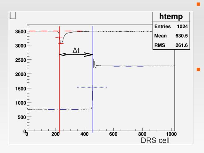
Trigger signal is sampled to correct for comparator jitter
