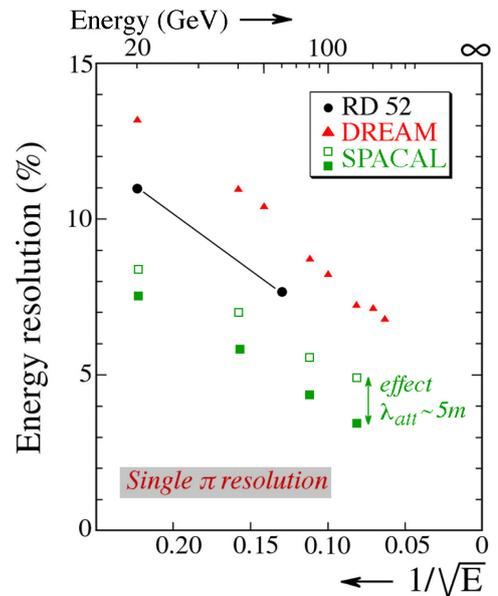
Figure 5: Comparison of the preliminary energy resolution obtained for single pions with the partially completed RD52 fiber calorimeter, and the published resolutions for single pions obtained with the DREAM calorimeter [2] and with the SPACAL fiber calorimeter [6]. The latter results are shown before and after correcting for light attenuation effects in the scintillating fibers.
