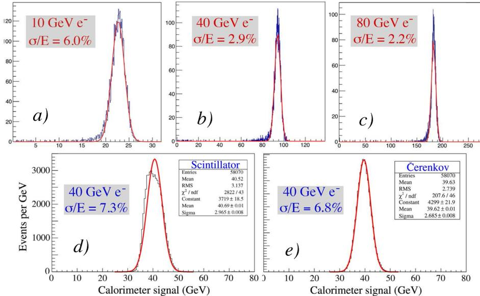
Figure 2: Response functions of the RD52 fiber calorimeter to electrons of 10 (a), 40 (b) and 80 (c) GeV, compared with the response functions of the DREAM calorimeter to 40 GeV electrons, in the scintillator (d) and Čerenkov (e) channels.
