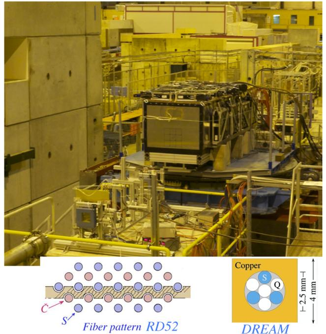
Figure 1: The partially completed RD52 fiber calorimeter during recent tests in the H8 beam line at the CERN SPS. The insert shows the fiber patterns in the RD52 calorimeter and in the original DREAM calorimeter.
