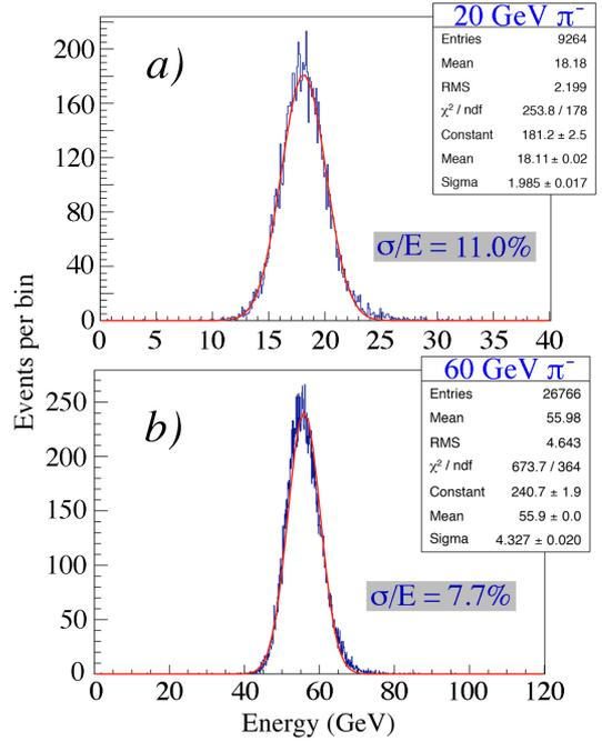
Figure 4: Preliminary response functions of the partially completed RD52 fiber calorimeter to 20 (a) and 60 (b) GeV  $\pi^-$ . No corrections for light attenuation and shower leakage were applied.
