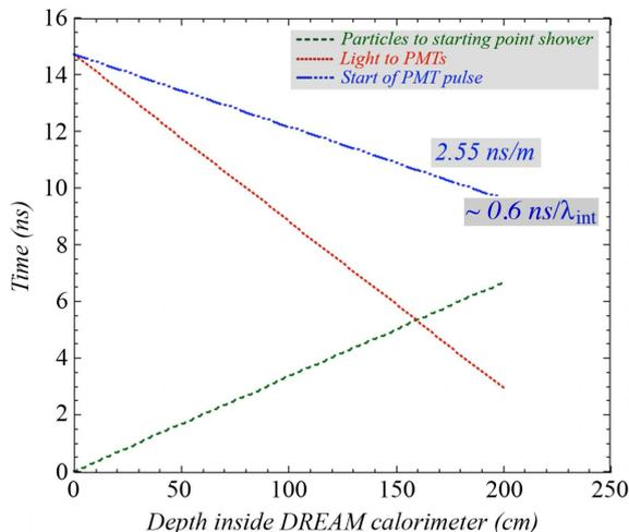
Figure 6: The dependence of the starting time of the PMT signals on the depth ( $z$ ) inside the calorimeter at which the light is produced. Also shown are the time traveled by the beam particles from the front face of the calorimeter to this depth  $z$  and the dependence of the time traveled by the light through the fibers from  $z$  to the PMT.
