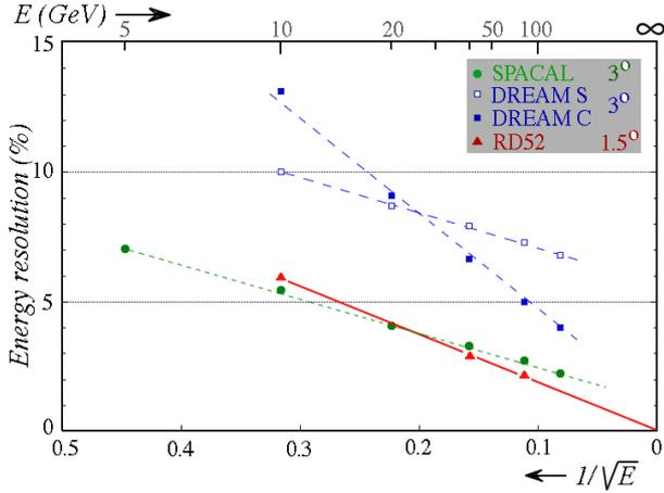
Figure 3: Comparison of the em energy resolution measured with the RD52 fiber calorimeter, the original DREAM calorimeter [5], and the SPACAL fiber calorimeter [6].
