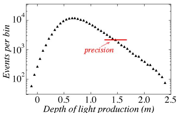
Figure 7: Event-by-event distribution of the depth at which the light is, on average, produced inside the calorimeter by the beam particles ( $60 \text{ GeV } \pi^-$ ).
