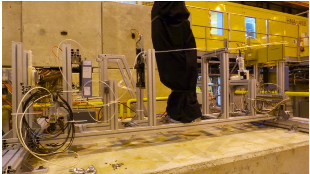
9 Pb modules (36 towers, 72 channels), 2 Cu modules (8 towers), 20 leakage counters (Plastic scintillator) 5
