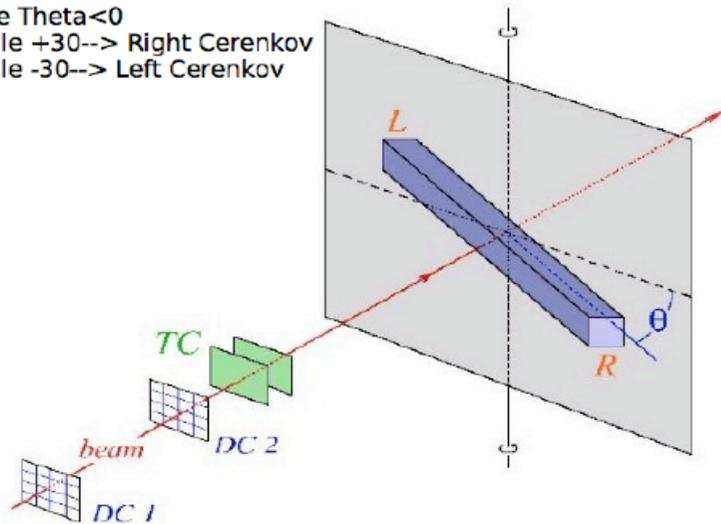
Single Crystal positioned on a rotating platform to perform angular scan
