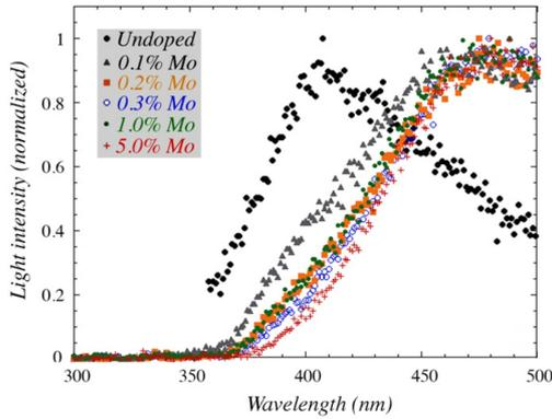
**Figure 1.** Normalized emission spectra for  $PbWO_4$  crystals doped with different fraction of Molybdenum, measured with radioluminescence.
