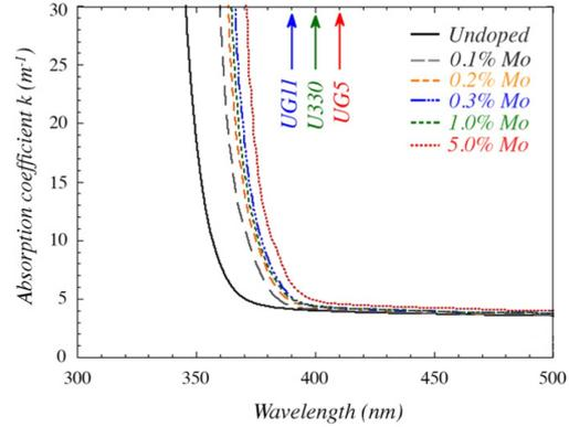
**Figure 2.** Absorption coefficient as a function of wavelength for  $PbWO_4$  crystals doped with different fraction of Molybdenum.
