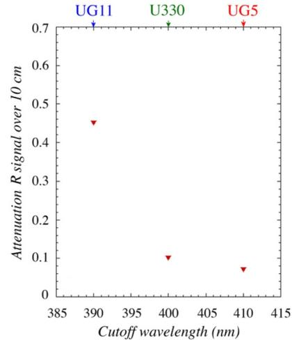
**Figure 6.** Relative change in the Cherenkov signal over a distance of 10 cm as a function of the optical filter cutoff in the  $PbWO_4$  crystals.
