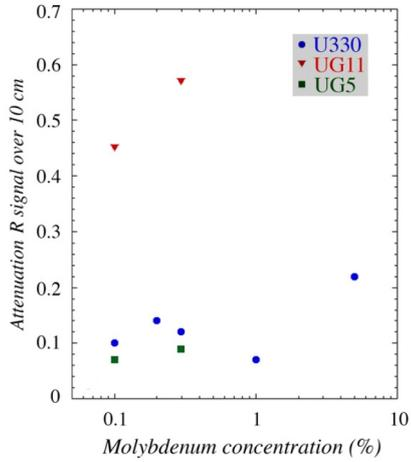
**Figure 5.** Relative change in the Cherenkov signal over a distance of 10 cm as a function of the Mo concentration in the  $PbWO_4$  crystals.
