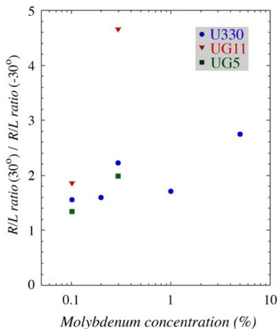
**Figure 3.** The ratio of the C/S signal ratios measured at  $30^\circ$  and  $-30^\circ$  as function of the Mo concentration.
