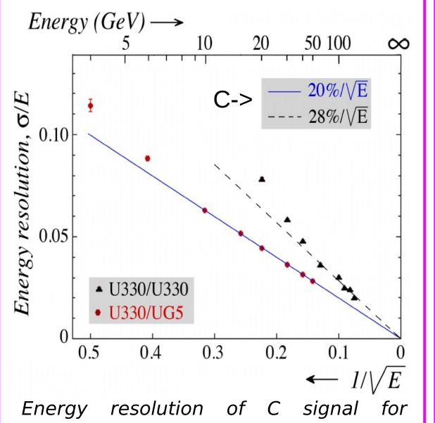
electrons showering in the crystal matrix, as a function of energy. Signal derived from different combinations of UV-filtered light detected at both ends of the crystal matrix.
