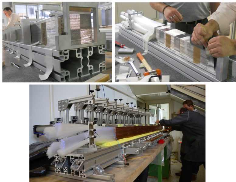
Figure 7. New SuperDREAM modules under construction at the University of Pavia (top), and at INFN Pisa (bottom). The Pavia modules use lead as absorber material, the Pisa ones copper.
