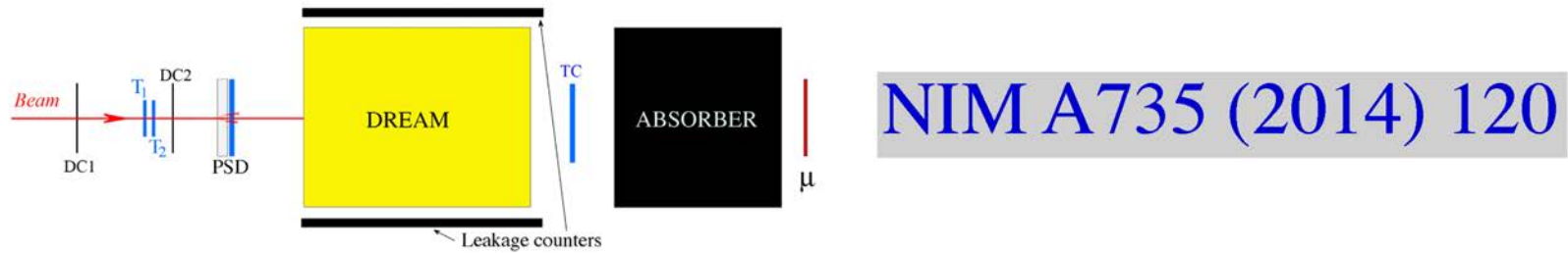
Fig. 4. Schematic overview of the arrangement of the auxiliary detectors that were used to identify the individual beam particles (not to scale). See text for details.
