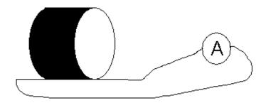
**a.** Determine which end of the cow magnet is north. Take a cow magnet and move it back and forth near the solenoid. Observe the ammeter while the magnet is moving.
