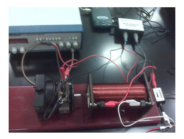
The function generator will be used to drive the oscillator back and forth. The driving wave function used will be a sine wave.
