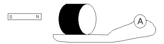
Put the north pole toward the loop. Then put the south pole toward the loop. Does the ammeter record a current? Which direction does the ammeter needle move when the north pole moves towards the magnet? Which direction does it move when the north pole moves away from the magnet? South pole towards? South pole away? Record your observations below.
