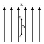
Calculate the potential difference between A and B in terms of E,  $x_1$  and any relevant angles.
