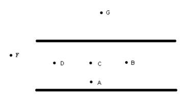
If the bottom plate is charged positively and the top plate is charged negatively, rank the values of the electric field at each of these points from highest to lowest. This is a prediction. (It is not right or wrong.) Each person in your group may make a different prediction.
