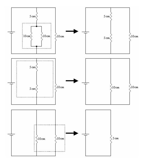
The network could be replaced by a single 5cm resistor.
