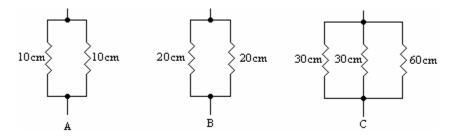
Each of these combinations is called a parallel network. Each of the parallel networks could be replaced by a single piece of nichrome wire that has the same resistance as the parallel network as shown in the figure below.
