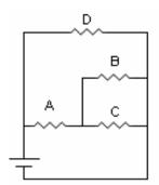
Suppose the current through resistor A is 1.5A, resistor B is 2.5A, and battery voltage is 1.5V. Find the resistance of each of the resistors: A, B, C, and D.
