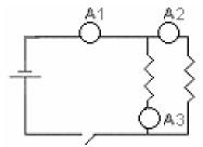
If the ammeter 1 reads 2.5 amps, and the nichrome wires are the same length what would ammeters 2 and 3 read? Explain your reasoning.
