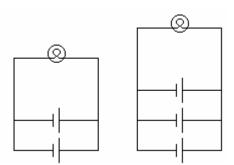
**a.** Compare the brightness of the bulb in each circuit to the brightness of a bulb in a circuit with one battery.
