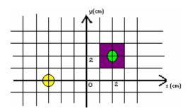
When we draw a grid, we choose where to put the origin of the grid. The position depends on where we choose to put the origin of the grid. We could represent the position of an object by an arrow from the origin of the grid to the location of the object. The position of an object at x = 7cm, y = 4cm is shown in the diagram below. It has a length of 8 cm and a direction 29.7° above the +x-axis.
