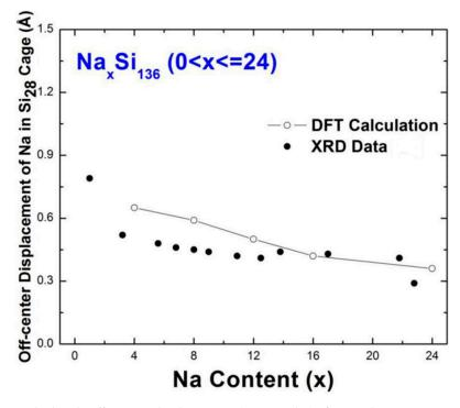
**Figure 5.** DFT-calculated "off-center" displacements (open circles) of Na in the Si<sub>28</sub> cages in Na<sub>x</sub>Si<sub>136</sub> as a function of Na composition (x = 4, 8, 12, 16, 24), along with XRD measured displacements (solid dots) by Beekman et al. [31].
