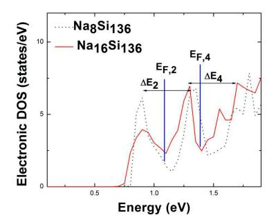
**Figure 1.** Illustration of the electronic density of states in the lower portion of the conduction band for clathrates Na<sub>8</sub>Si<sub>136</sub> and Na<sub>16</sub>Si<sub>136</sub>. The Fermi energy levels ( $E_{F,2}$ ,  $E_{F,4}$ ) are marked by blue lines and quasi-activation energies  $\Delta E_2$ ,  $\Delta E_4$  are given regarding sharply peaked structures.
