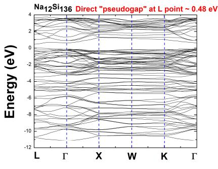
Figure 2. Electronic band structure of Na<sub>12</sub>Si<sub>136</sub>.
