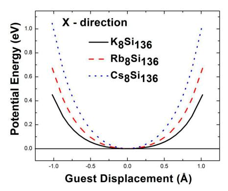
**Figure 6.** The potential energy curves for alkali atoms K, Rb, and Cs inside the Si framework. X represents the motion direction with respect to the alkali atom.
