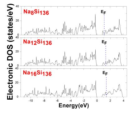
**Figure 3.** Electronic density of states (DOS) of the clathrate system  $Na_xSi_{136}$ , where x = 8, 12, 16. The Fermi energy levels ( $E_F$ ) are denoted by dotted lines.
