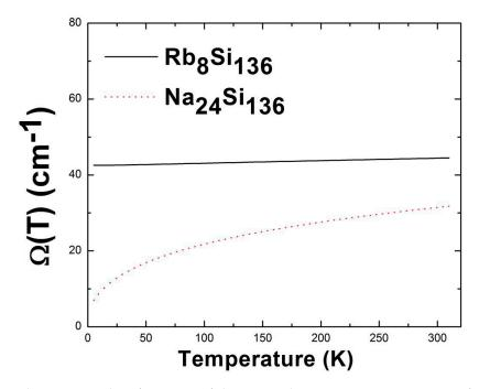
**Figure 7.** Anharmonic rattling frequency of the guest vibrations in an  $Si_{28}$  cage as a function of temperature for the filled binary clathrates  $Rb_8Si_{136}$  and  $Na_{24}Si_{136}$ .
