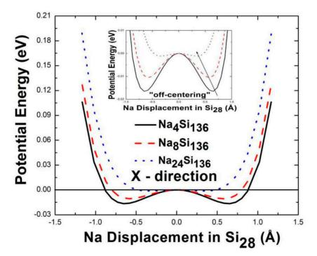
**Figure 4.** The calculated isotropic Mexican-hat shaped potential-energy curves for Na vibrations in the large 28-atom cages in the clathrate system  $Na_xSi_{136}$  (x = 4, 8, 24). X represents the motion direction with respect to the Na atom.
